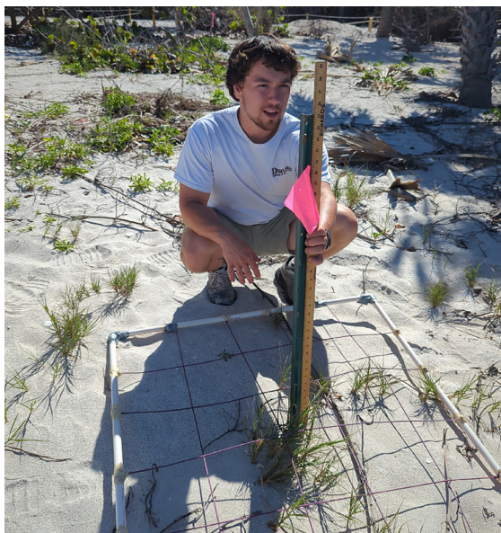
FGCU student Tristan Dumas installs a metal spike that will track how much sand plants accumulate.
